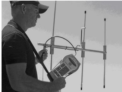
Tracking a Seasafe Personal Transmitter signal using Seasafe Receiver and Directional Antenna (note: the antenna is held in the vertical plane). Receiver is being used in the portable mode with the optional rubber protection holster and neck-strap
