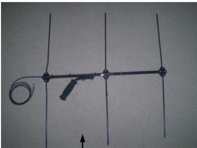
"directional-antenna" unfolded for use
